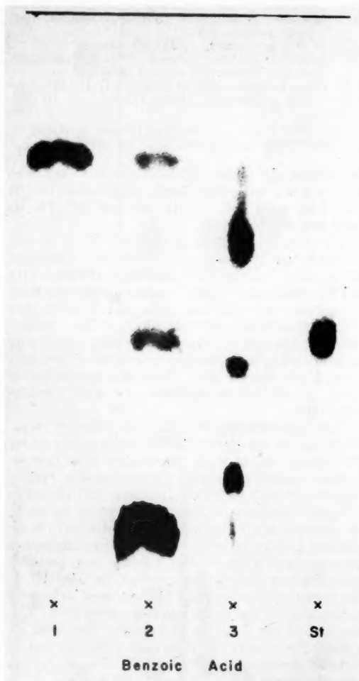
FIG. 3. Radioactive metabolites of C^{14} -carboxyl-labeled benzoic acid from pea epicotyls. Radioautographs of chromatograms of tissue extracts: 1) ether extract at pH 7.0; 2) ether extract at pH 2.6; 3) n -butyl alcohol extract at pH 2.6. (St.) is a marker of radioactive benzoic acid. The mobile, neutral substance ( R_f 0.75 in 1 and 2) is chromatographically indistinguishable from benzamide. The slow moving acidic substance ( R_f 0.14 in 2) is benzoylaspartic acid.
